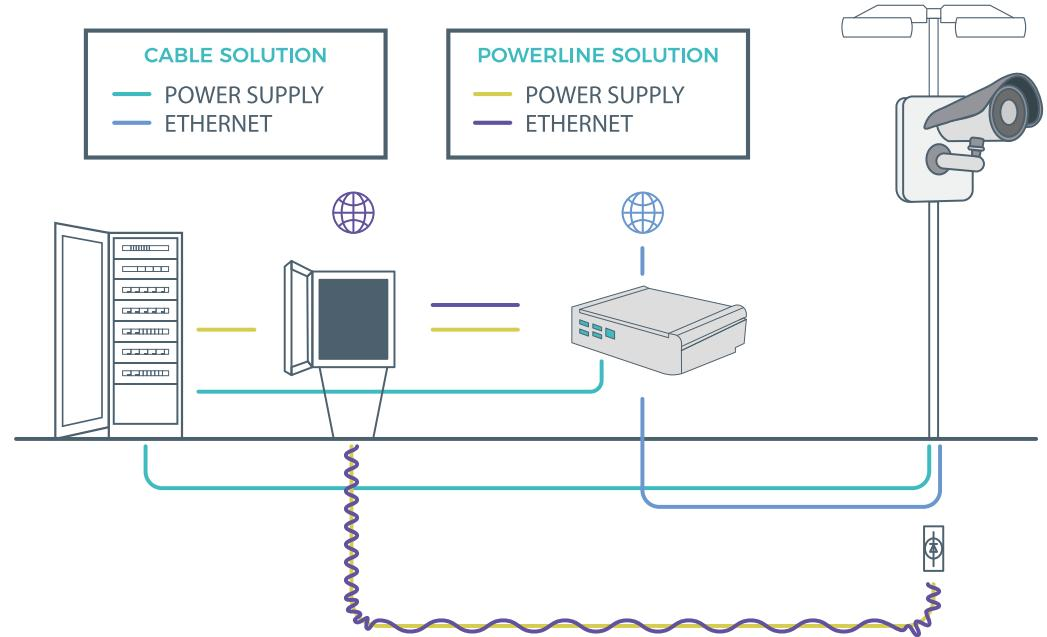
Park smart system could be installed next to camera or, with an additional kit based on powerline, close to the electrical panel that supply cameras. The unique qualities of Park Smart are:
